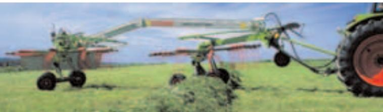
Maximum working width or maximum overlapping. The cylinder can be switched to a second bore. Simply select your desired position.
