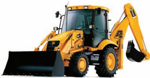
Backhoe Loader 3CX
